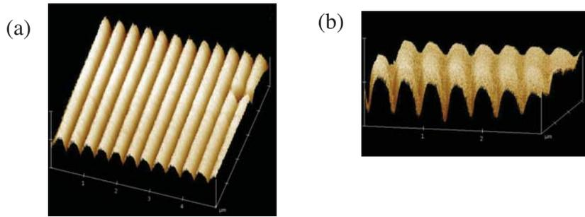
**Figure 3.** Atomic-force microscopy analysis of the fringes written by multiphoton absorption into PMMA.
