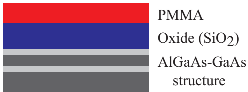
(3) Spin-coat e-beam resist
