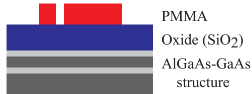
(4) Pattern inverse with e-beam & develop
