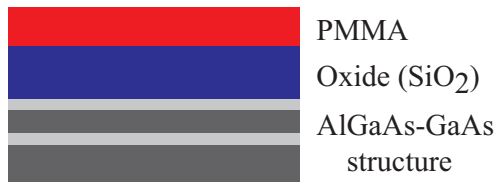
(3) Spin-coat e-beam resist
