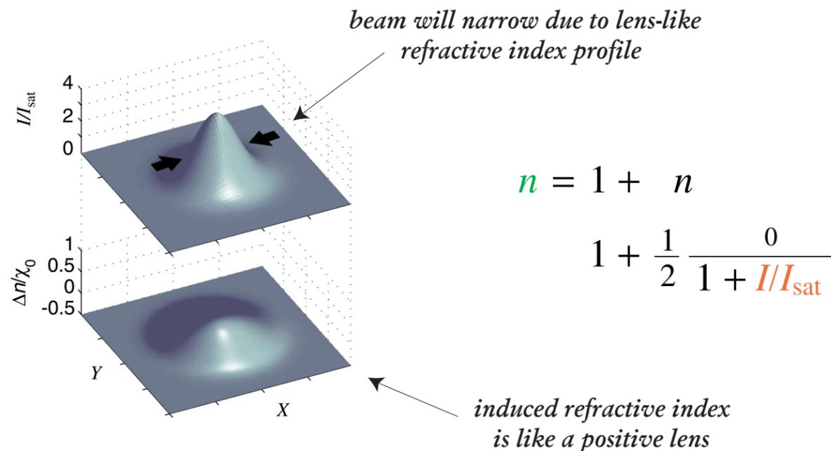
Since light refracts in the direction of increasing index, in a medium with negative saturable nonlinearity it refracts toward regions of higher intensity. This causes smooth beams to narrow or **self-focus**. But it also tends to destabilize a beam as small amplitude fluctuations grow due to local self-focusing. Thus beams with even small amplitude noise can spontaneously split into two or more separate beams.
