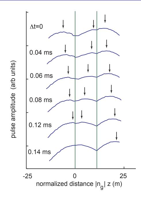
Observation of Backward Pulse Propagation in an Erbium-Doped-Fiber Optical Amplifier
