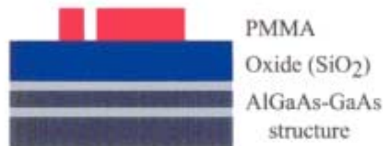
(4) Pattern inverse with e-beam & develop
