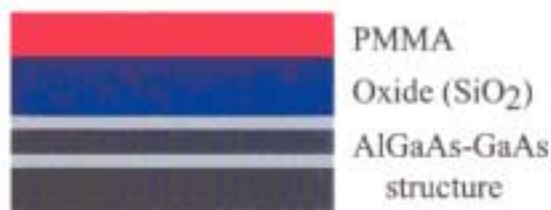
(3) Spin-coat e-beam resist
