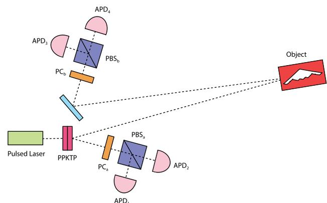
FIG. 5. Schematic for a proposed secure time-of-flight experiment, based on the entanglement-based Ekert QKD protocol. Polarization-entangled photon pairs generated in a pair of crossed PPKTP crystals are used to measure the distance to an object. Security against an intercept-resend jamming attack is checked by carrying out a test for a CHSH Bell inequality with measurements in appropriate polarization bases using PC and PBS.
