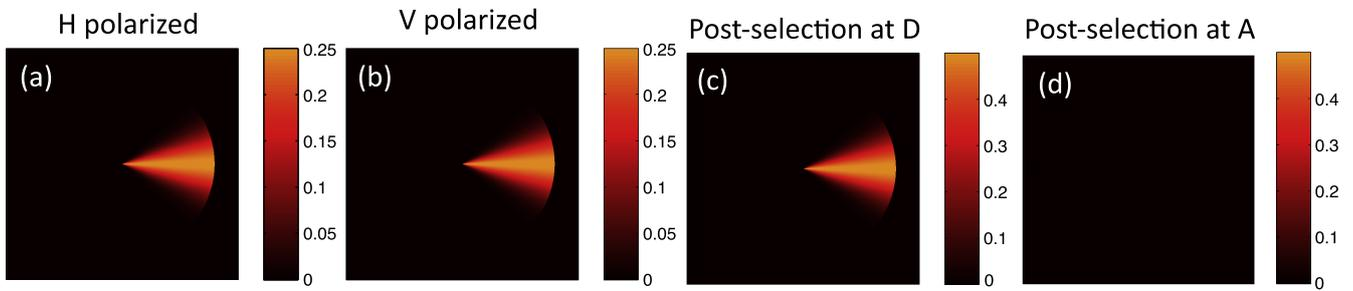
**Figure 3.** Simulation results. (a) Shows the spatial profile of the Gaussian wedge in one of the arms of the interferometer. The polarization of this beam is aligned in the horizontal direction. (b) Shows the vertically polarized beam in the second arm. (c) Shows constructive interference when the position of the post-selection polarizer set diagonally. (d) Shows destructive interference when the post-selection polarizer is anti-diagonal.
