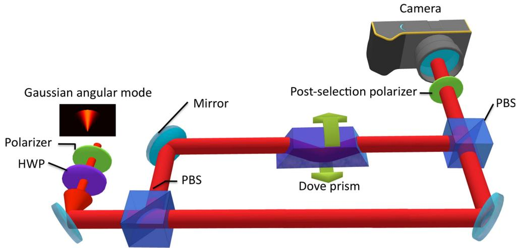
**Figure 2.** Experimental setup. An angular wedge is prepared in diagonal polarization by means of a polarizer and half wave plate (HWP). The beam is split by a polarizing beam splitter (PBS) and rotated by a Dove prism, the beam is rotated by twice the angle of the Dove prism. A post-selection polarizer is used to amplify the rotation induced by the Dove prism.
