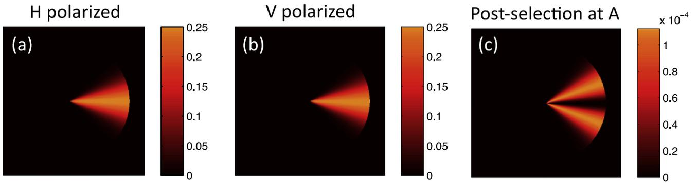
**Figure 4.** Simulations of a small rotation. The horizontally polarized beam (reference) in one of the arms of the interferometer is shown in (a). The vertically polarized beam is rotated by  $0.5^\circ$ , this is shown in (b). (c) The intensity after an anti-diagonal post-selection polarizer.
