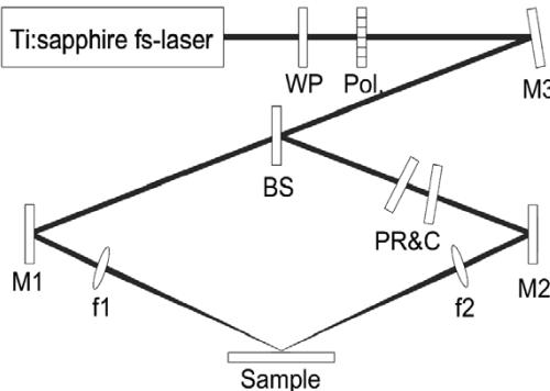
Figure 4. Experimental set-up. WP, half-wave plate; Pol., polarizer; M1,M2,M3, mirrors; BS, beam splitter; f1,f2, lenses; PR&C, phase retarder and compensator.
