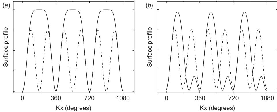
Figure 2. Theoretical surface profile for various experimental parameters. (a) Solid curve is for  $N=3$ ,  $M=1$ ; dotted curve is for  $N=3$ ,  $M=2$ . (b) Solid curve is for  $N=3$ ,  $M=2$  and the phase shift of the second shot is  $\pi + \Delta$  ( $\Delta = \pi/3$ ); dotted curve is for  $N=3$ ,  $M=2$ , and the phase shift of the second shot is  $\pi$ .
