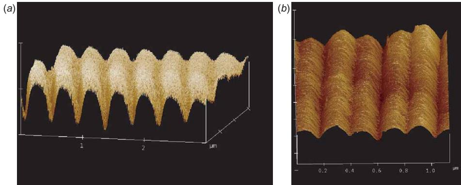
Figure 5. AFM images of the fringes recorded on a PMMA film. (a) Result for a single exposure, leading to fringes with a period of 425 nm. (b) Results for a sequence of two exposures, leading to a period of 213 nm.
