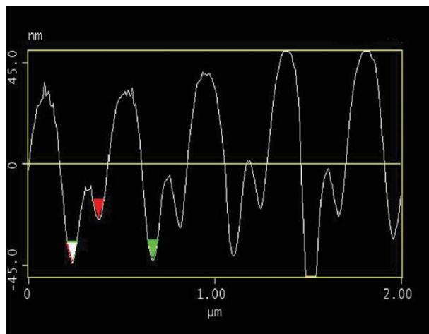
Figure 6. Surface profile of the non-sinusoidal fringes. In this case, we shifted the phase of the second shot by  $\Delta = \pi/3$ .
