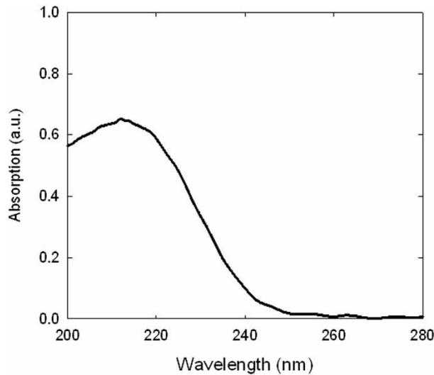
Figure 3. The UV absorption spectrum of the PMMA film.
