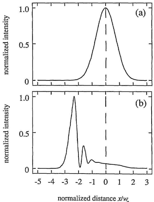
Fig. 3. Results of a numerical simulation of the transverse intensity profile of the probe beam (a) before and (b) after it copropagates with the pump beam through the sodium cell.
